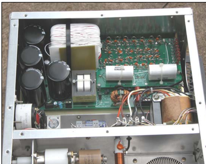
This shot shows the PS-2500A high voltage switching power supply. The white thing at top left is the high voltage transformer. The two HV output caps are center right; total output "C" is .2 mf at 4000 VDC.
