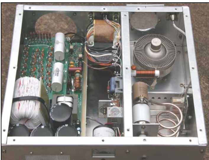
Top view, showing Watts Unlimited PS-2500A switching power supply at far left. The center section is the control circuitry, including filament transformer, time delay relay and metering. The RF compartment is on the far right.
