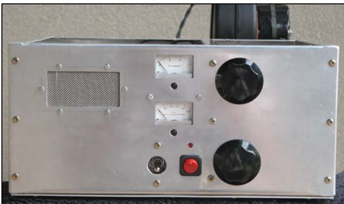
Front view, showing exhaust port on left, plate current meter top center grid current meter at center, recessed power switch and amp in/out switch with LED indicator above. Top removable knob upper right is plate tune; lower removable knob is plate loading. Air intake for power supply is on bottom of cabinet. RF compartment is pressurized so that 95% of air exhausts thru anode cooler and the rest exits thru the cathode compartment.
