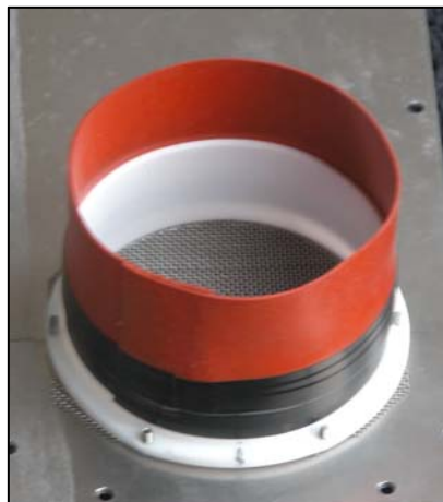
Teflon chimney with rubber "extension" for pressurizing anode compartment
