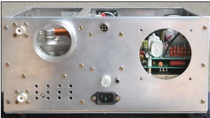
Rear view, showing RF input and output connectors at bottom left and top left; mounting flange for blower, cathode compartment air exhaust (under blower flange), AC power connector for blower and fan upper center, fuse, RCA PTT, and AC mains connector, hole for muffin fan at far right. Both openings are "screened" with stainless screening.
