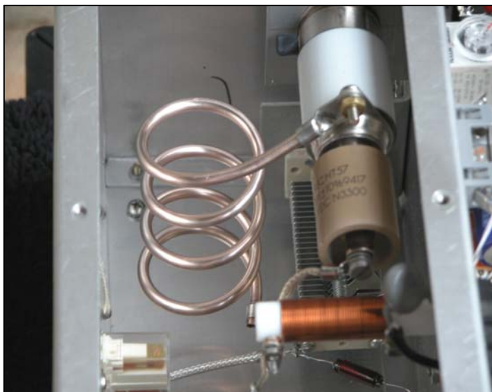
Larger view of tank circuit, showing silver-plated tank coil, 3-30 vacuum variable, 857 blocking cap, RF plate choke and almost buried at the bottom, the 200 pf loading cap.
